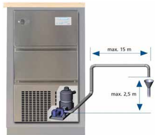
Fig. 6: Principal illustration of application with optional condensation water pump.
